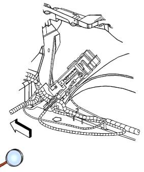
5. Align the module to the vehicle antenna module bracket.
